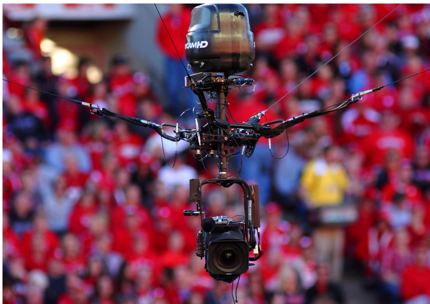
Obr. 1.8: Systém SKYCAM pre polohovanie kamery [3]
