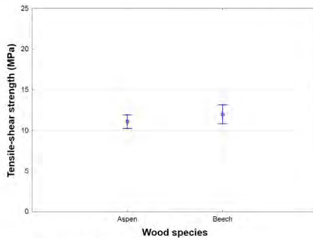
Fig. 2. Influence of wood species on tensile-shear strength
