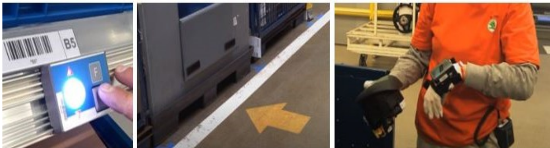
Obr. 2.7 Pick To Light, Pick To Point a Pick To Voice
