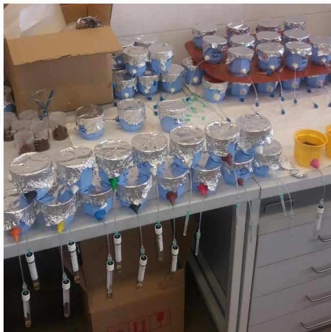
Figure 5: Pore water collection with rhizon samplers after incubation period
