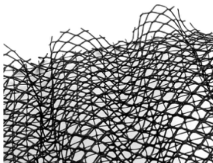
Obr. 8: 3D georochož (PP/HDPE/PET) (Geomat, 2017)
