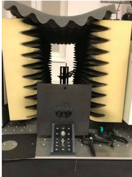
Figure 23: Dark room with experimental instrument for measuring retroreflectivity and holder
