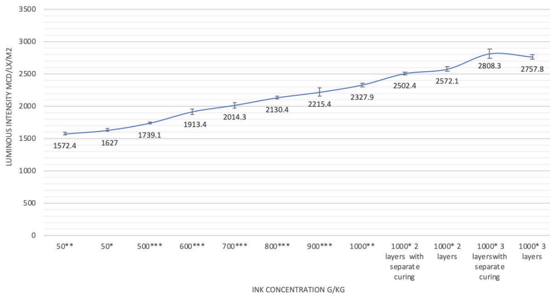
Graph 4: Relationship between average and upper/lower CI 95% for navy blue sample 45° right side
