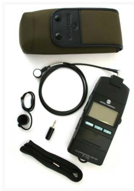
Figure 22: The Konica Minolta T-1 Illuminance Meter [42]
