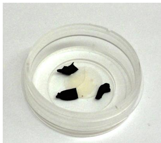
Figure 22 A sample prepared for ISO 10993-5 biological test
