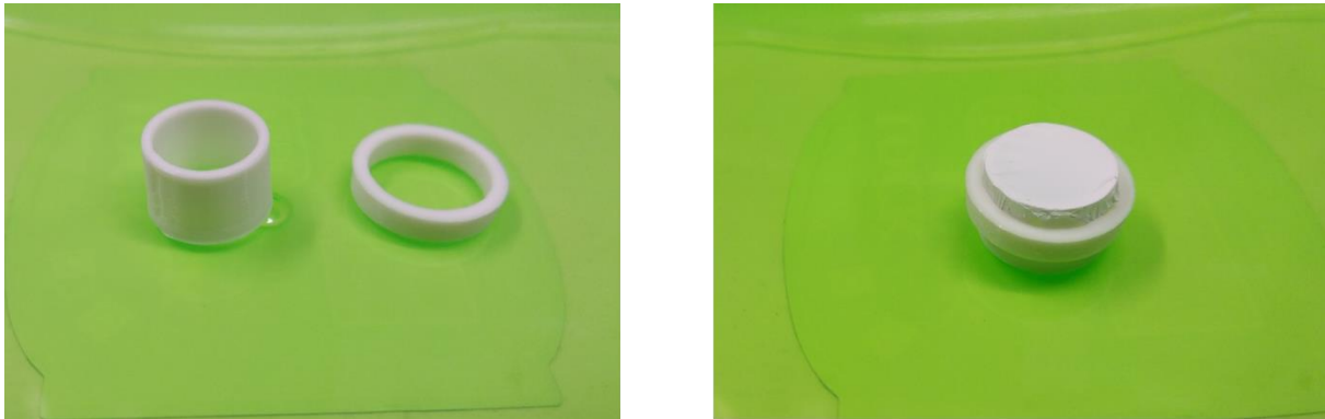
Figure 21 Sample holder for the SBF test, a) empty holder; b) holder with a sample
