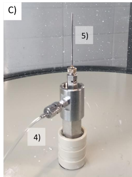
Figure 18 a) 4Spin (Contipro, Czech Republic); b) electrospinning setup: 1) syringe with the precursor, 2) emitter, 3) collector; c) detail of the emitter: 4) precursor supply tube, 5) needle
