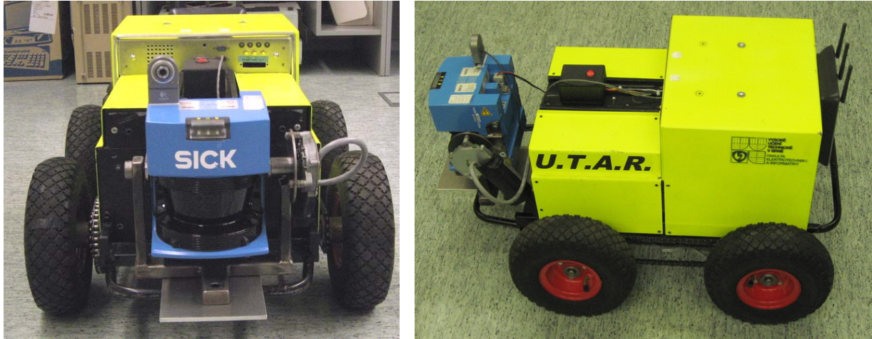
Figure 10: The U.T.A.R. robot with continuous inclining device
