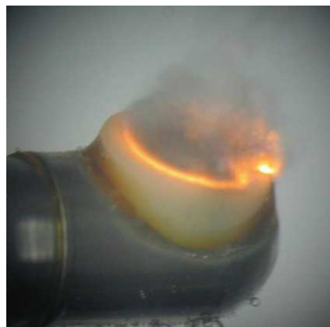
Figure 46 The detail of power electrode structure with plasma under liquid (yellow area).
