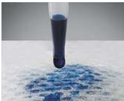
Figure 8 Plasma treatment of hydrophilises fabrics and technical nonwovens by jet technology [11].
