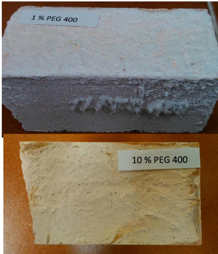
**Fig. 54** Geopolymer mortar specimens containing 1 and 10 % PEG 400.
