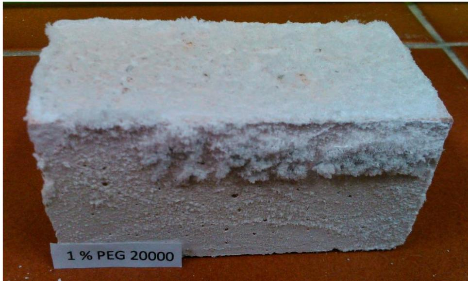
**Fig. 56** Geopolymer mortar specimens containing 1 % of PEG 20000.
