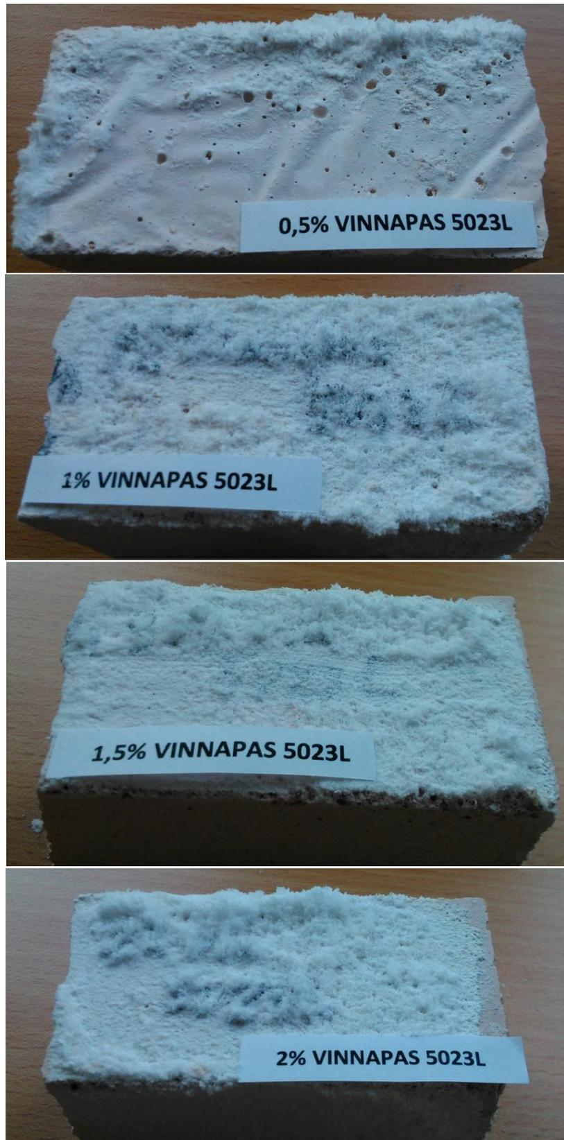
**Fig. 58** Geopolymer mortar specimens containing 0.5, 1, 1.5 and 2 % of Vinnapas<sup>®</sup> 5023 L.
