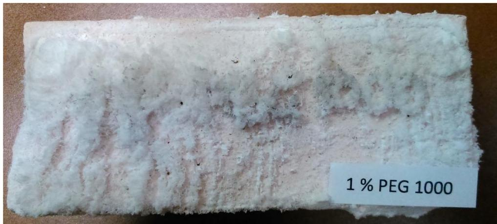
**Fig. 53** Geopolymer mortar specimens containing 1% PEG 1000.
