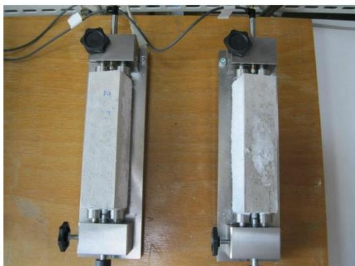
Fig. 17 Measuring the linear shrinkage of AAS mortar specimens.
