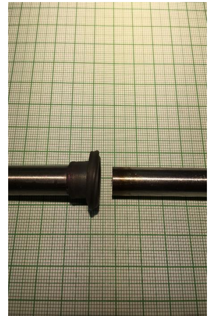
Fig. 56 Cracked friction weld after tensile test
