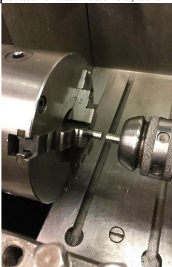
Fig. 39 clamping of welded materials
