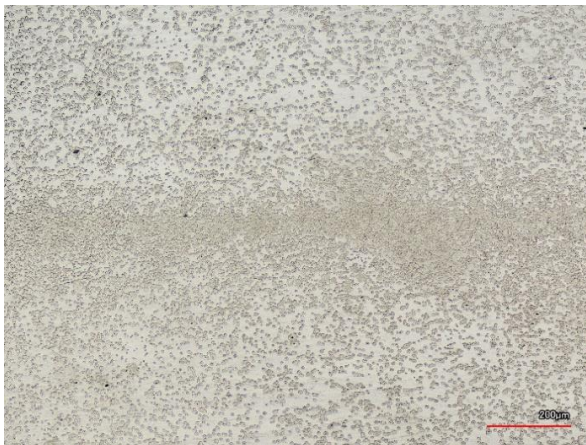
Fig. 49 Microstructure of AISI 316L weld (10x zoom)
