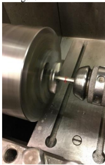
Fig. 40 Contact of welded materials
