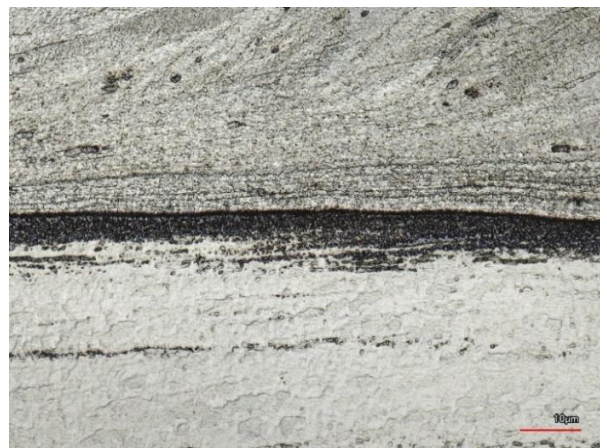
Fig. 52 Microstructure of AISI 316L and Ti GR2 weld (150x zoom)
