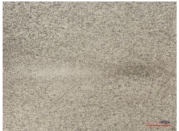
Fig. 50 Microstructure of Ti GR2 weld (10x zoom)
