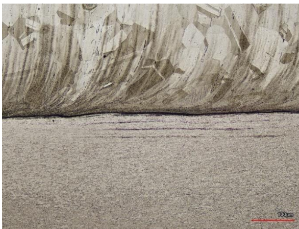
Fig. 51 Microstructure of AISI 316L and Ti GR2 weld (20x zoom)
