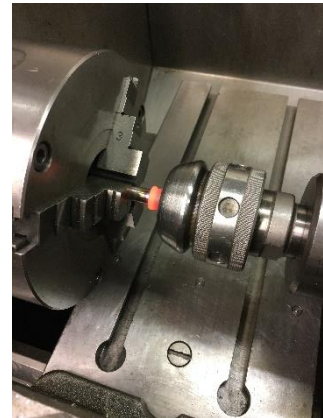
Fig. 43 application of forging pressure
