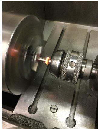
Fig. 42 forming suitable weld
