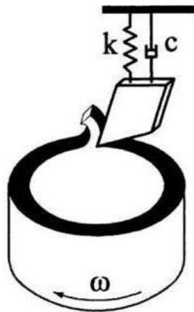
Picture 1. Model of regenerative chatter
