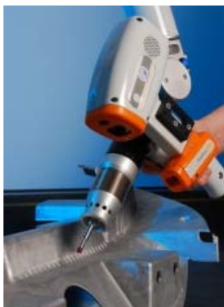
Obr. 2.6 ModelMaker skener MMD 26
