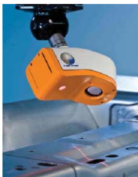
Obr. 2.2 Laser skener LC60D 22
