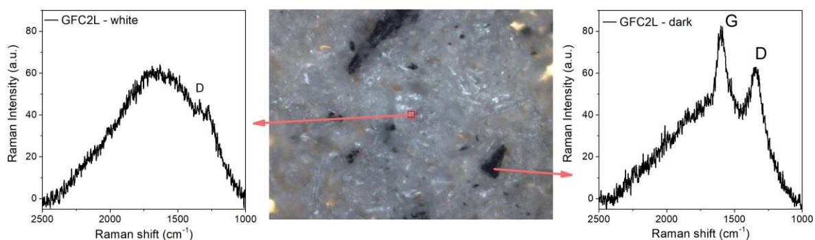
Figure 15: Raman spectra of GFC2L recorded on two crystals differing in color.
