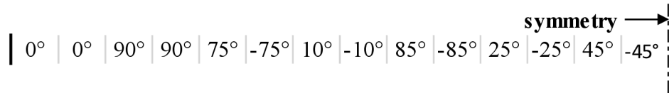
Fig. 4.1 Stacking sequence coding of a laminate
