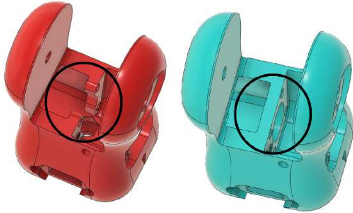
Figure 5.8: The modified link 4 (red) and the original part (blue)
