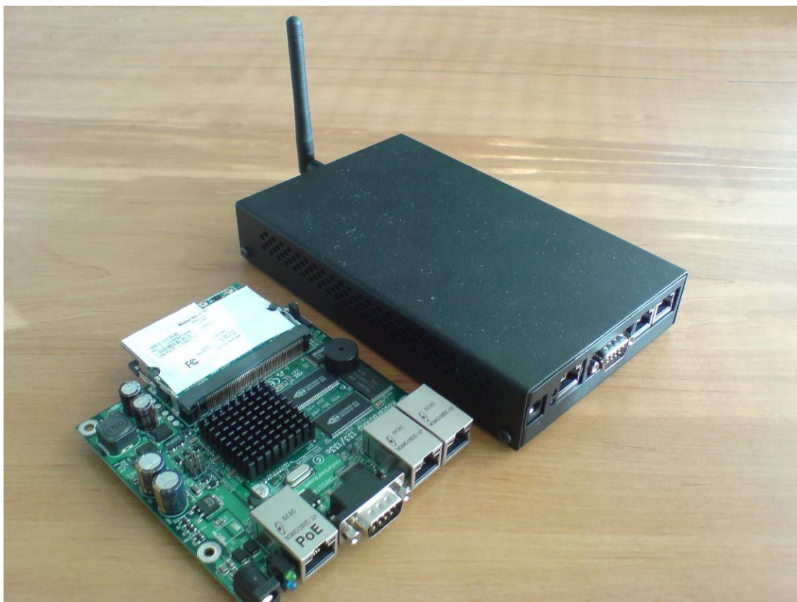
Obr 6.1: HW platforma Mikrotik RouterBoard 133.
