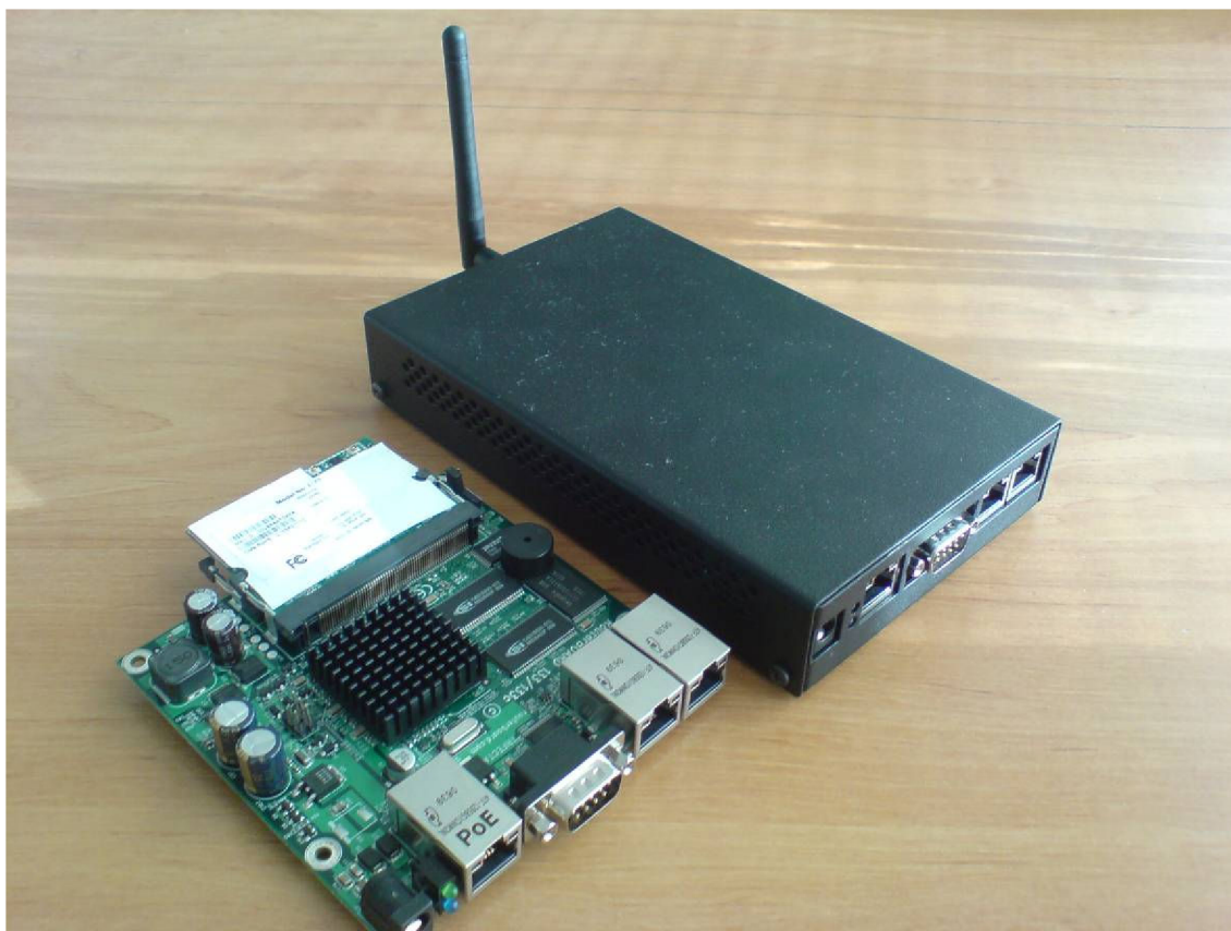
Obr 6.1: HW platforma Mikrotik RouterBoard 133.
