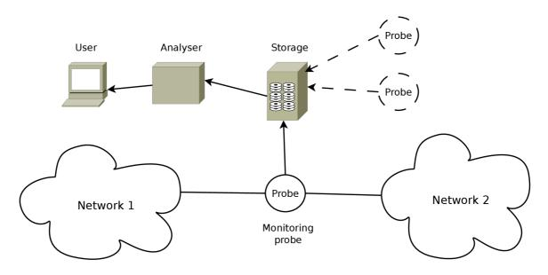
Figure 2.3: Schema of a monitoring system architecture.
