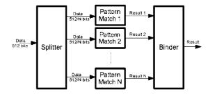
Fig. 1. Increasing the throughput by multiple pattern matching units.
