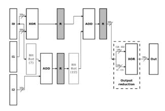
Fig. 5. Pipelined implementation of NSGAHash6.
