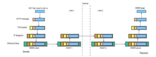
Figure 2.1: Example of the data encapsulation on the Sender side and the data decapsulation on the Receiver side.
