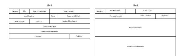
Figure 2.2: Comparison of IPv4 header (left) and IPv6 header (right).
