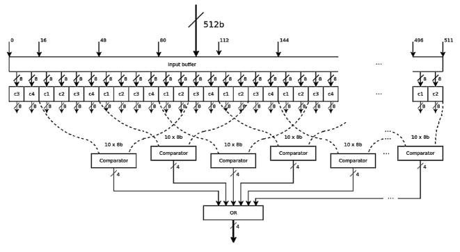
Fig. 3. Classifier CL-acc as a combinational circuit.
