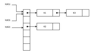
Fig. 1. Hash table with separate chaining.
