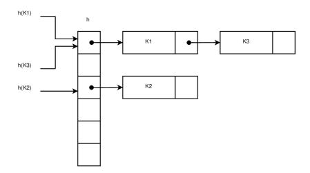
Figure 2.8: Example of hash table with size 6 slots, utilizing the separate chaining.
