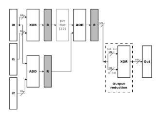
Fig. 4. Pipelined implementation of NSGAHash5.
