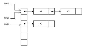
Figure 1: Hash table with separate chaining.
