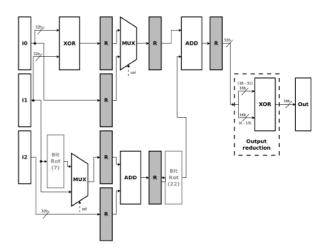
Fig. 6. Reconfigurable hash function RecoHash.
