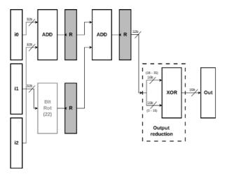
Fig. 3. Pipelined implementation of NSGAHash4.
