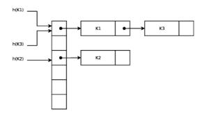
Fig. 1. Hash table with separate chaining.
