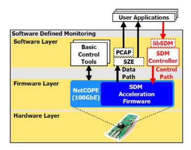
Figure 2.4: Software Defined Monitoring system architecture (adopted from [43]).
