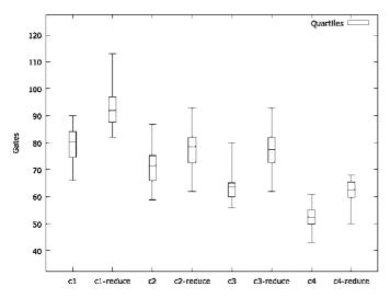
**Fig. 5.** The number of gates obtained at the end of 20 CGP runs for four coders (c1, c2, c3 and c4) of classifier CL-acc. 'Reduce' stands for 'reduced set of gates'.
