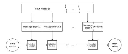
Figure 2.7: Merkle–Damgård construction of hash functions.
