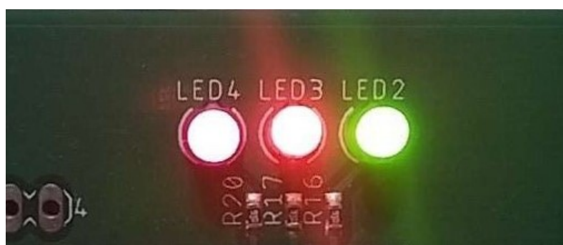
Obr. 7.5: LED 2, 3 a 4 na cievkach 29, 30 a 31
