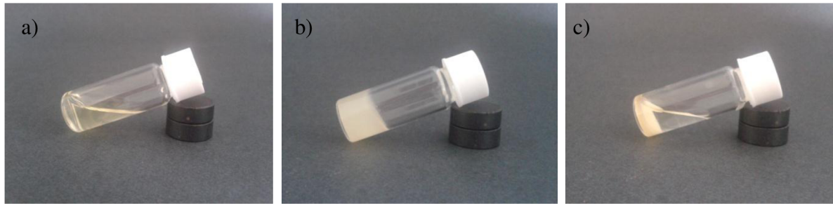
Figure 52 Inverting test tube method: a) the solution in phase sol b) the phase gel at 37 °C, c) the phase suspension.
