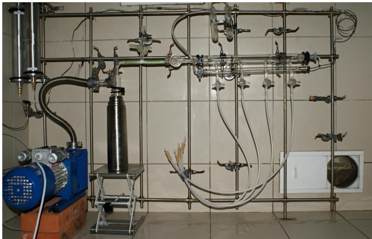
Figure 34 Vacuum line-manifold for experiments under inert atmosphere in Polymer Synthesis Laboratory at Faculty of chemistry BUT.
