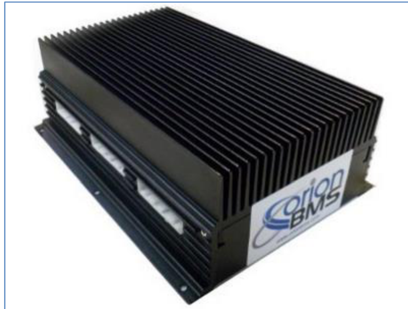
Image: Battery control module (Orion BMS)
