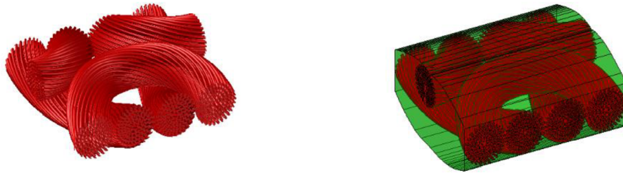
Figure 6.6. A volume enclosing the repeat of the knitted fabric structure.
