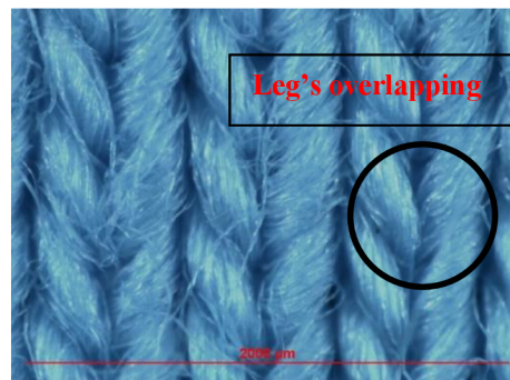
(h) Microscopic image of legs overlapping at SWP 4% and 35 Ne
