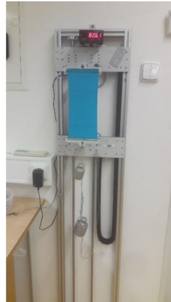
Figure 4.7. Applied tension force
