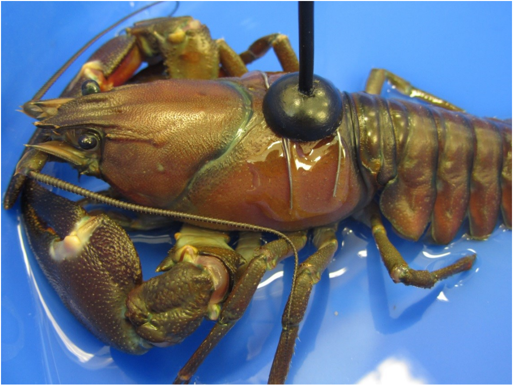
Fig. 2.7. Photo of the crayfish with attached NIR optical sensor.
