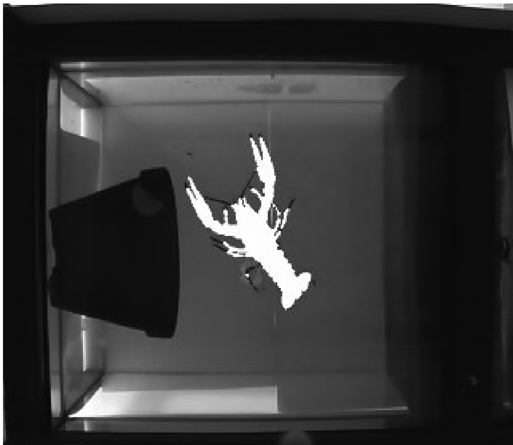
Fig. 2.5. Example of moving crayfish detected on the camera image. The image pixels classified by the motion detection algorithm as belonging to moving object are marked with white color.
