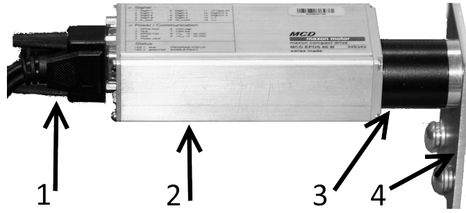
Figure 2: Drive train. 1-serial port connection, 2-Maxon MCD EPOS 60W stepper motor, 3-planetary reduction gear head Maxon GP 32 C, 4-mount plate (the body of inspection device).
