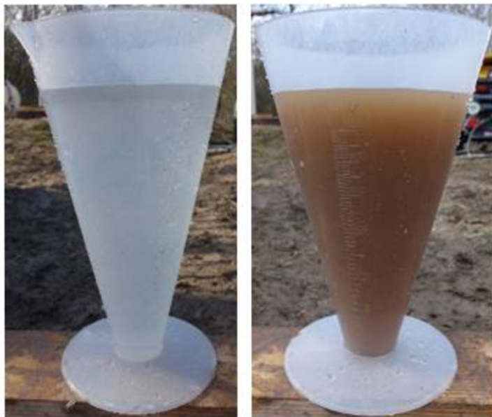
Figure 9. Comparison of turbidity in raw water before (a) and after the start (b) of ultrasound rehabilitation.
