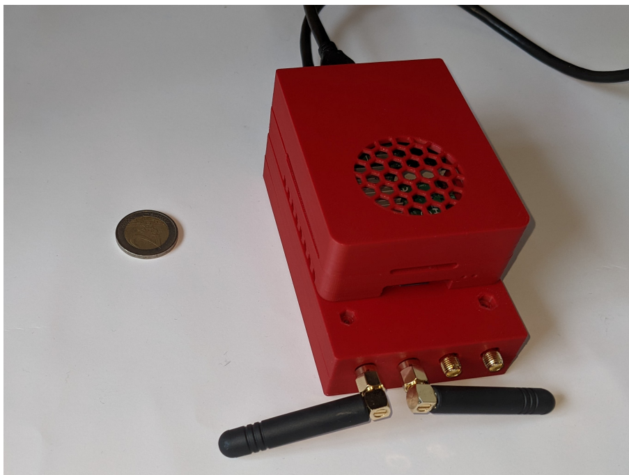
Figure 4.2: Our chosen hardware - Raspberry Pi 4B+ and BladeRF Micro 2.0 AX9. Both enclosed in 3D printed Case.
