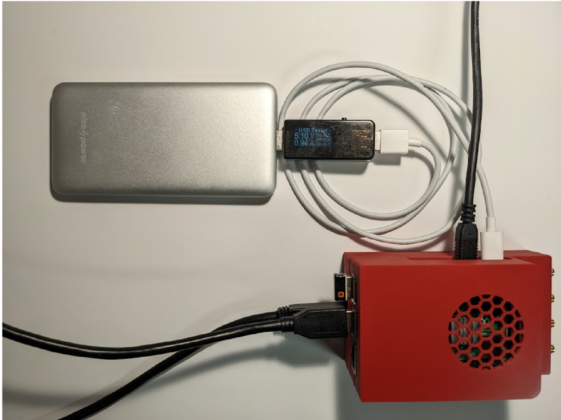
Figure 6.1: Running the setup on the battery. We were able to run BladeRF without second power bank.
