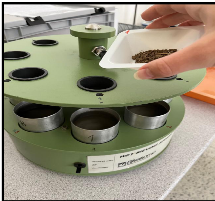
Obr. 6: Wet sieving apparatus (autor, 2022)
