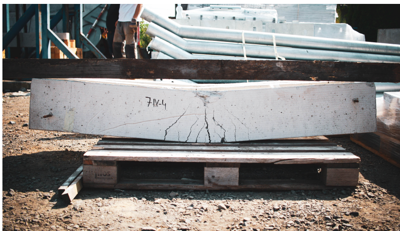
Fig. 8.2. Damaged specimen 7IX-4 after the impact.
