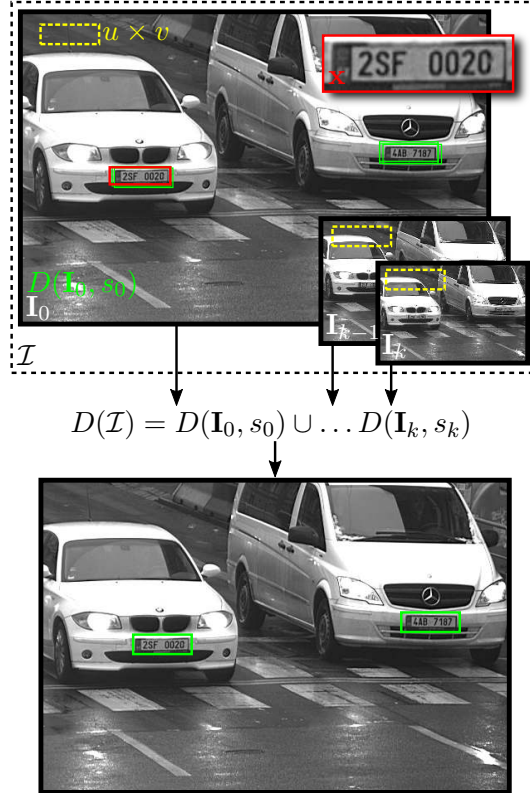
Figure 5.2: (top) The detection process on pyramidal image representation \mathcal{I} . The detection window of size u \times v (yellow), is used for classification of every position m, n in image (example in red). The result of detection on each image is a set of locations D(\mathbf{I}, s) accepted by the classifier (green). (bottom) The final detection result after non-maxima suppression.
