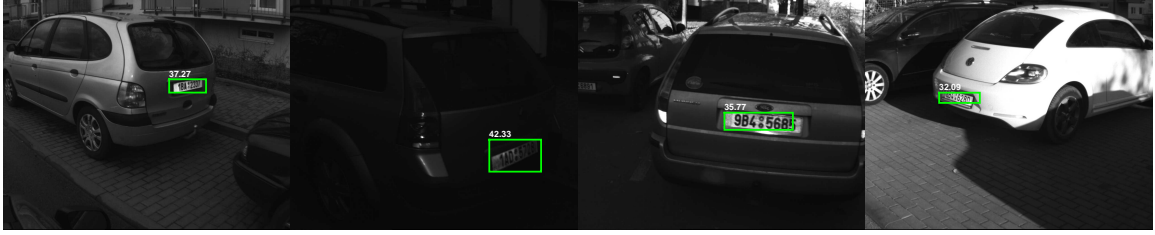
Figure 6.1: We detect license plates in wide variety of deformations in challenging light conditions. The images show the detected license plates with a confidence value.
