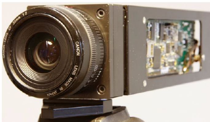
Figure 7.3: The camera prototype using OnSemi CMOS image sensor and Xilinx Zynq SoC.
