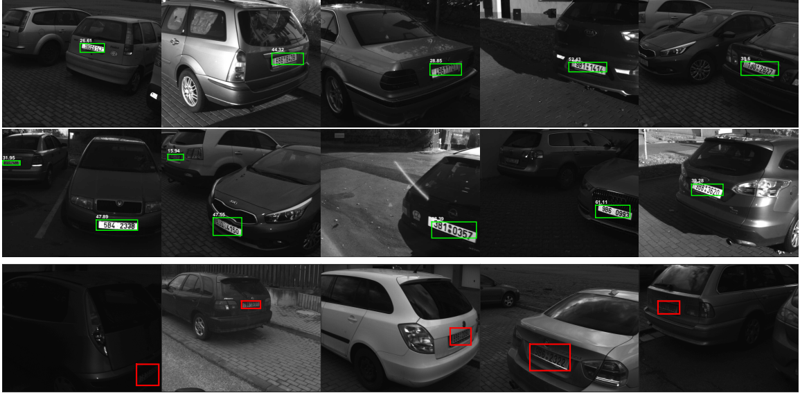
Figure 6.6: (top) Examples of detected license plates and detector responses. (bottom) Missed license plates (annotations marked by red).
