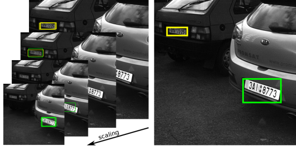
Figure 6.2: (left) Image scales and objects detected by the classifiers. (right) Final detections after non-maximum suppression. The classifiers are color-coded, the yellow one detects license plates almost aligned, the green one detects slightly tilted license plates.
