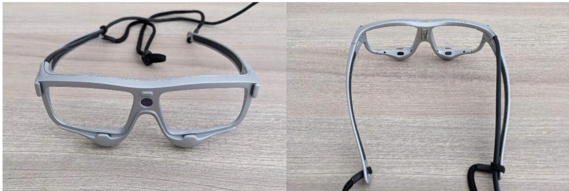
Figure 7. SMI eye tracker glasses.
