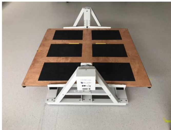
Figure 4. Stabilometer (model 16030, Lafayette Instrument, Indiana, IN, USA)
