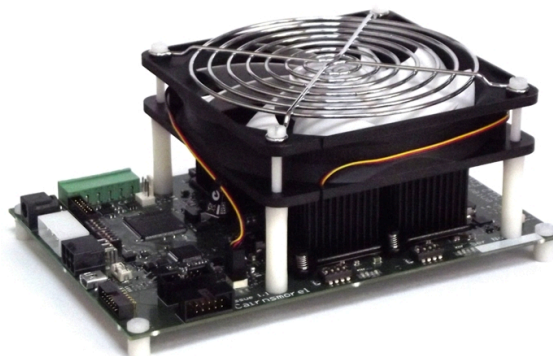
Figure 4: FPGA card modified for bitcoin mining [source: enterpoint.co.uk]
