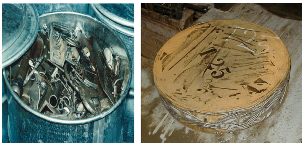
Fig. 15 Drum filled with the waste, and the drum after high-pressure molding (UJV Rez, 2008b).
