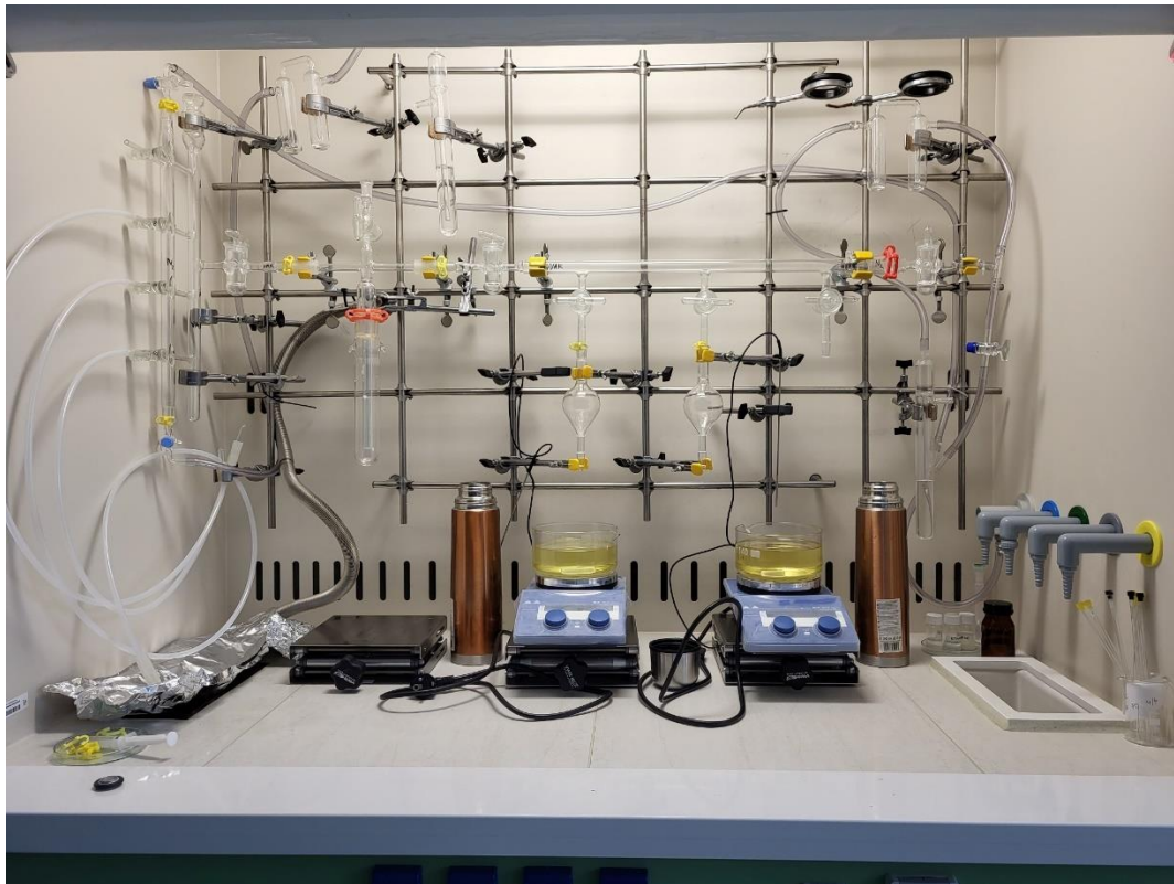
Figure 13: Vacuum line for copolymer synthesis.
