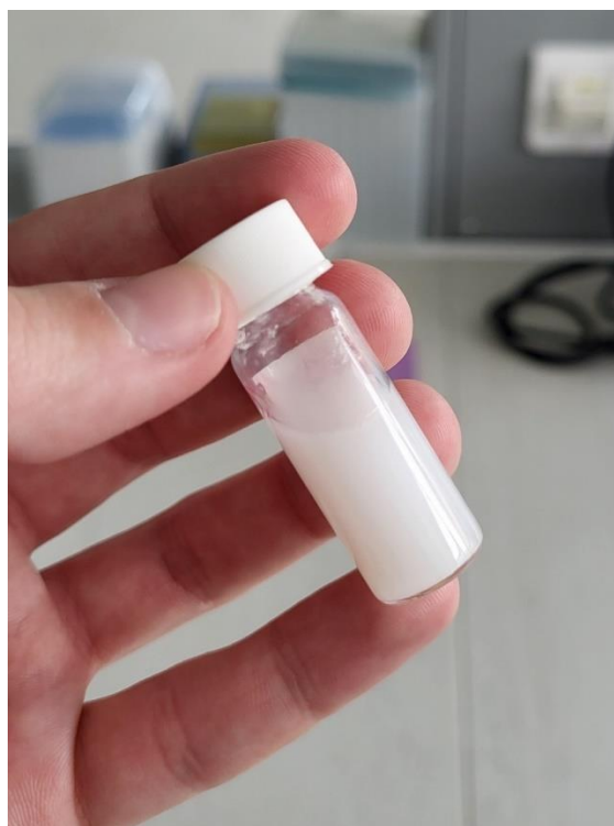
Figure 15: Copolymer solution - dissolved copolymer in the required solution after 4 days of stirring in the refrigerator.
