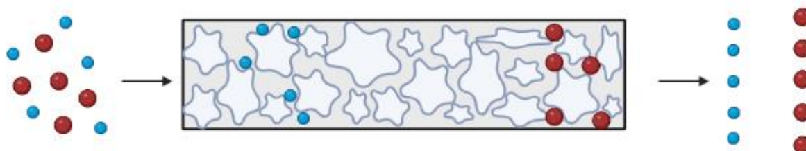
Figure 18: GPC technique for separating dissolved molecules according to their size [12].
