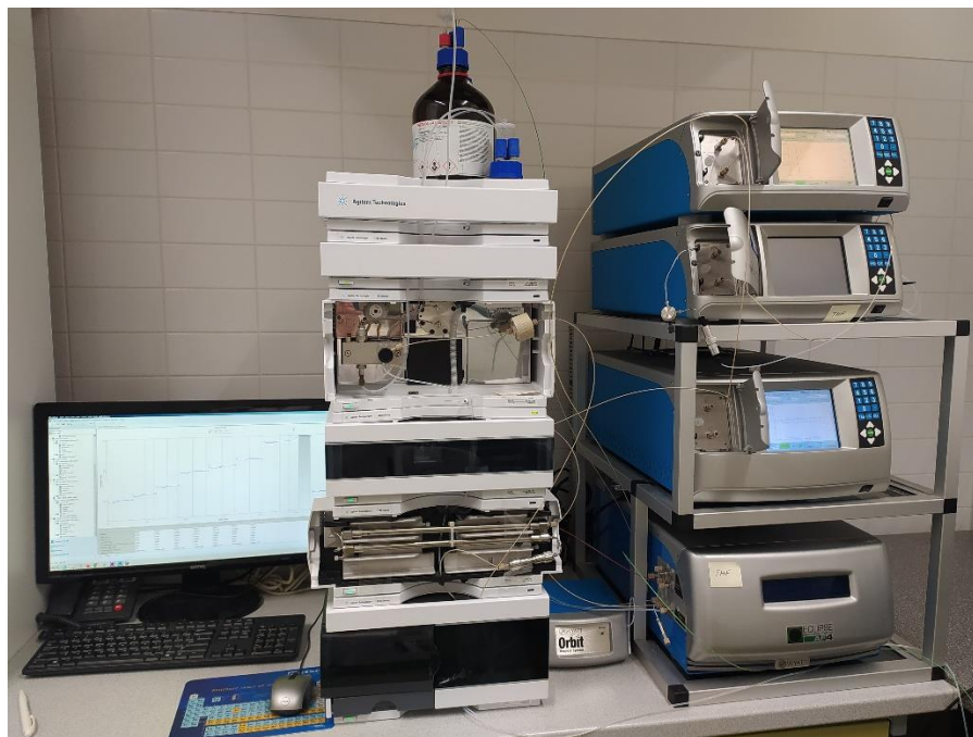
Figure 19: Gel permeation chromatography GPC/SEC system 1260 Infinity with Multi-Angle Light Scattering (MALS) photometry DAWN HELEOS II.
