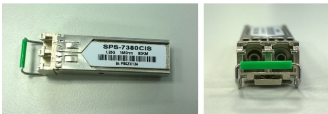
Obr. 6.5: SFP modul SPS-7380CIS
