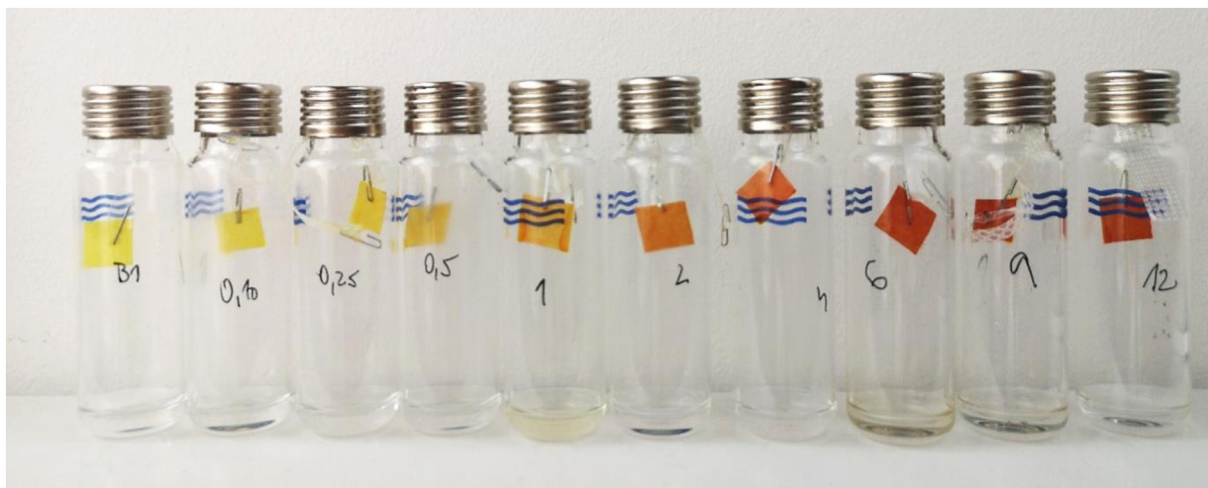
Figure 11: Colour change of picrate paper strips observed when samples were taken out from the oven after 20 hours.
