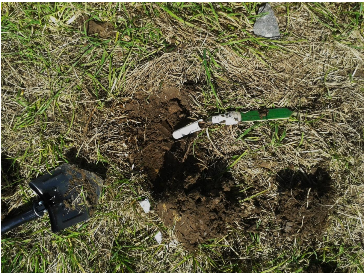
Fig. 4 A sensor destroyed after being ran over by a tractor.
