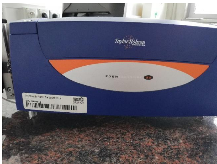
Obr. 28: Drsnoměr Form Talysurf Series Intra 2
