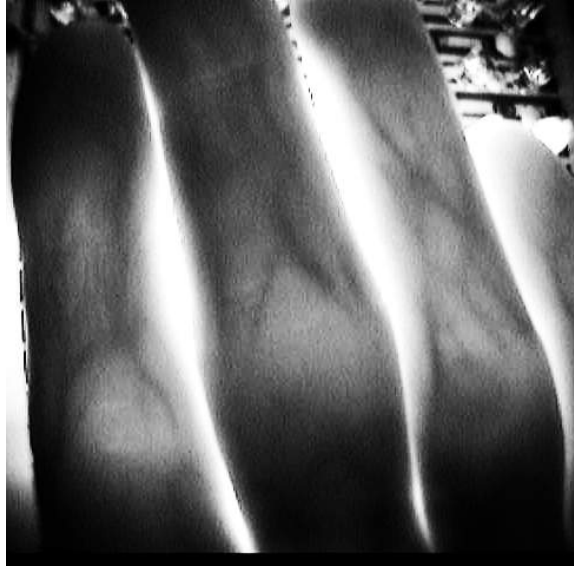
Figure 1.8: Surface vein detection using NIR.
