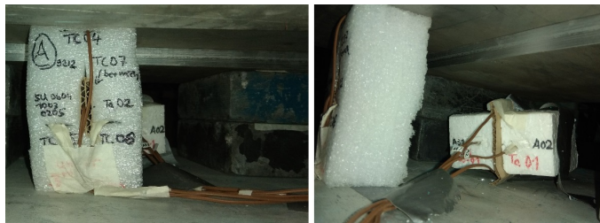
Figure 4.32: Neutron leakage setup for under the QUINTA target measurement. On the left side is displayed the insulation box with samples under the third section. On the right side, there is shown a similar measurement under the second section where was expected larger neutron flux. It was expected to measure sharp but small temperatures change caused by direct heating of n leakage fission reactions due to thick insulation which suppress the heat transfer from the QUINTA target. These photographs show the measurement setup before the final position fixation, so it looks orderless.
