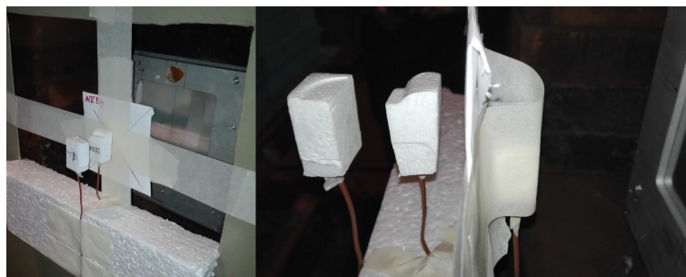
Figure 3.25: Proton beam online monitoring by proton reactions heating probes.
