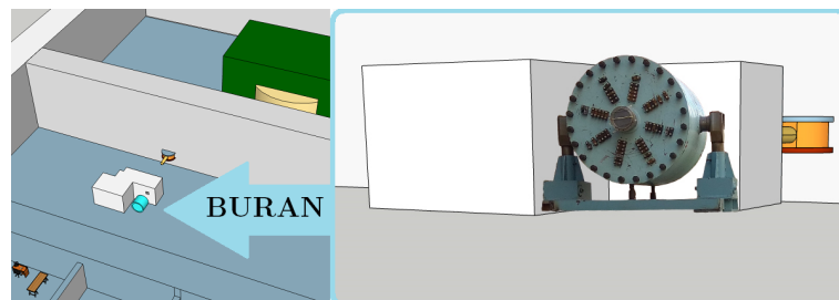
Figure 2.11: Sketch of the experimental hall with BURAN sub-critical blanket, on the right side enlarged view with collage of real photograph. Compare this figure with sketch of already performed experiments disposition shown on Fig. 3.1 where all parts description is given. The 3D Inventor model of the BURAN is available for download in appendix on p.197, item No. 6.
