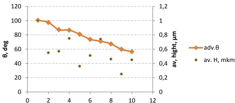
**Figure 11.** Decreasing of contact angle compare to the surface roughness.
