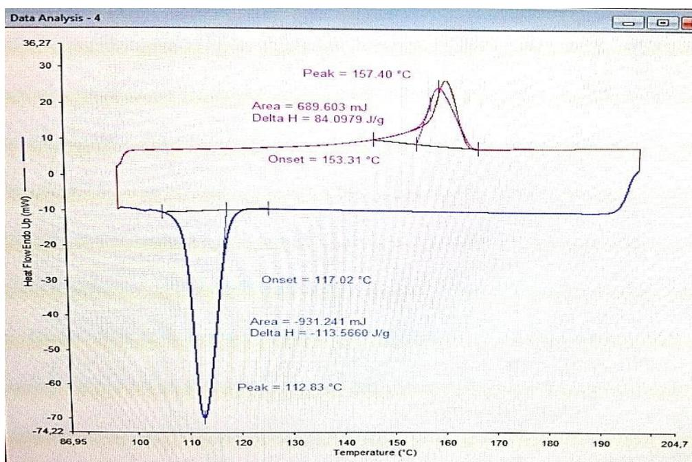
**Figure 3.** Reresulted DSC thermogram. The first heating-cooling cycle was carried out to erase thermohistory of sample preparation. The result of the second heating was taken for calculation.
