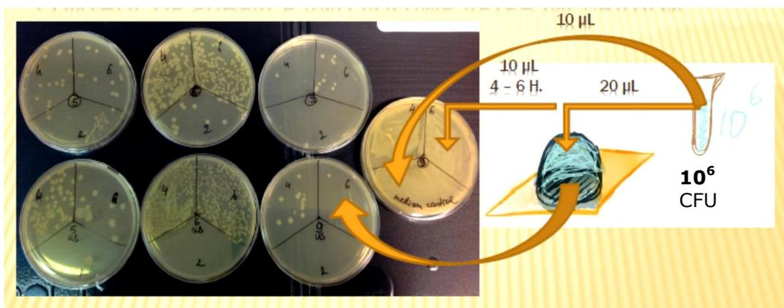
**Figure 14.** This experiment shows no bactericidal activity of composition in the bacterial suspension in contact with polymer surface. Number of bacteria cells counted from 10 µl of the medium cultivated 6h on the sample N<sup>o</sup>9 is the same as in initial medium, cultivated in flask during the same time. However the same sample composition N<sup>o</sup>9 prevents the bacteria cells attachment to the polymer surface (bacteria survive, but not form a monolayer).
