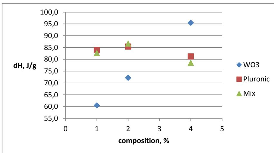
**Figure 4.** Melting enthalpy as the function of wt% of individual components.
