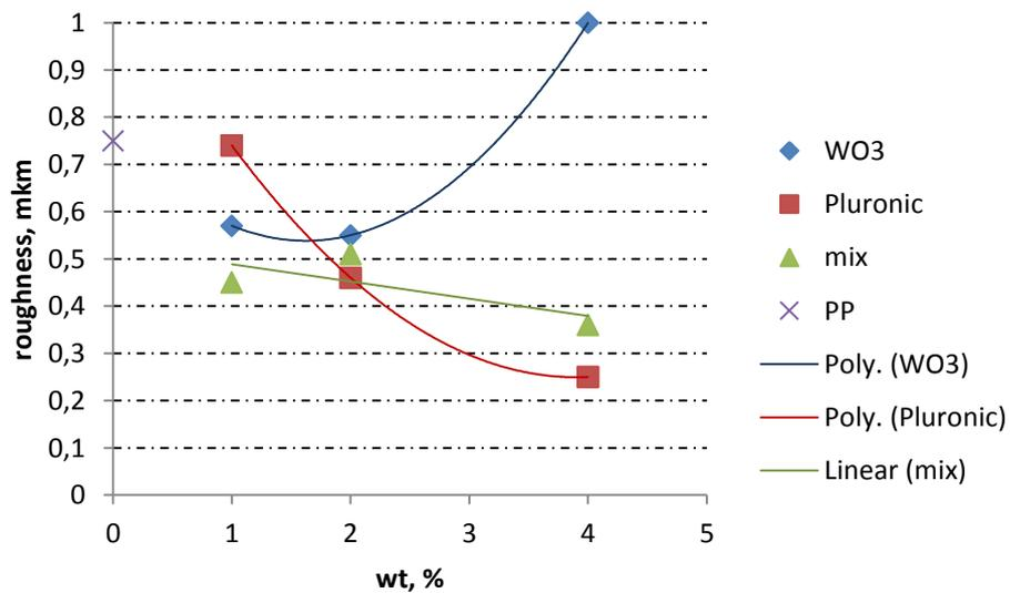
**Figure 10.** The influence of components on the surface roughness.
