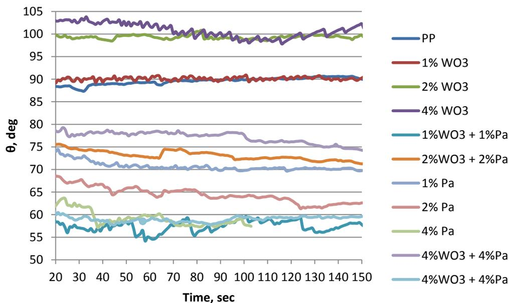
**Figure 6.** Wetting properties of polypropylene modified with  $\text{WO}_3$ , Pluronic and the mixture of both. Static angle of 2  $\mu\text{l}$  water drops (lower upper panel) on the samples and advancing (0.1  $\mu\text{l}/\text{sec}$ ) water contact angle (lower panel).
