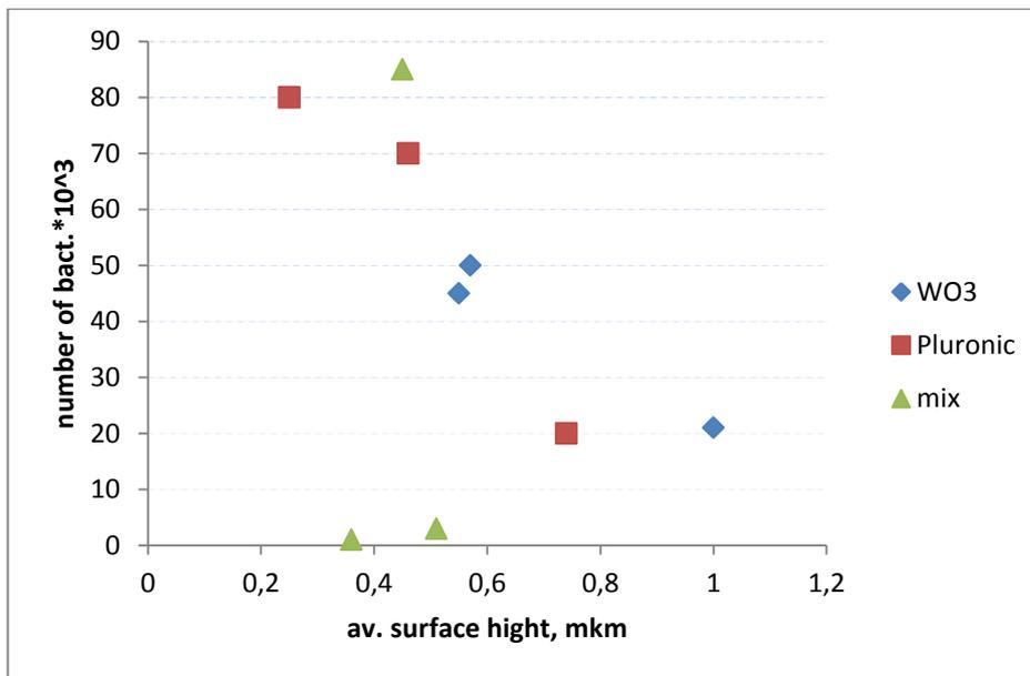
**Figure 18.** Number of bacteria adhered cells as a function of roughness of different surfaces. There no visible influence of surface roughness on antimicrobial activity. Presented data support earlier statement that topology of surfaces can be neglected.
