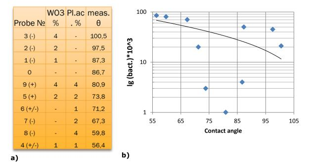
**Figure 17**. Measured contact angle (a). Number of bacteria cells adhered on different surfaces as a function of contact angle and composition (b).
