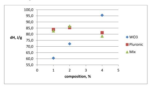
**Figure 4**. Melting enthalpy as the function of wt% of individual components.
