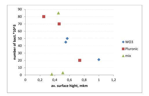
**Figure 18.** Number of bacteria adhered cells as a function of roughness of different surfaces. There no visible influence of surface roughness on antimicrobial activity. Presented data support earlier statement that topology of surfaces can be neglected.
