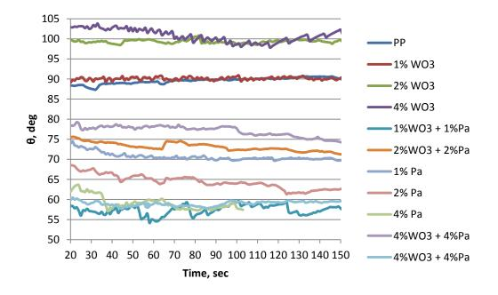
**Figure 6.** Wetting properties of polypropylene modified with WO3, Pluronic and the mixture of both. Static angle of 2  $\mu$ l water drops (lower upper panel) on the samples and advancing (0.1  $\mu$ l/sec) water contact angle (lower panel).
