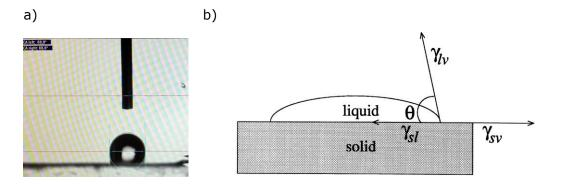
**Figure 5**. Snapshots of water droplet on the layer formed by water and polypropylene (a). Contact angle formed by a liquid at the three phase boundary where a liquid, gas and solid intersect (b).
