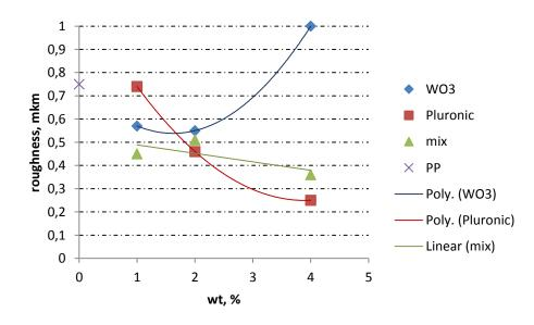
Figure 10. The influence of components on the surface roughness.
