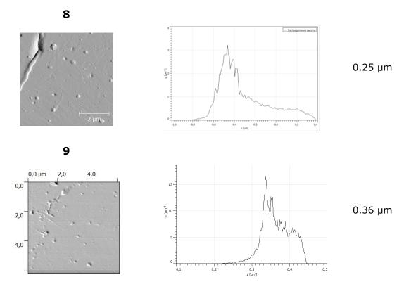
**Figure 9.** AFM images of PP samples and average roughness (profile amplitude) calculated from AFM
