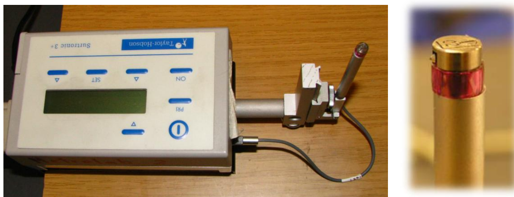
Fig. 4.8 - Stylus instrument with a skid pick-up and a tip
