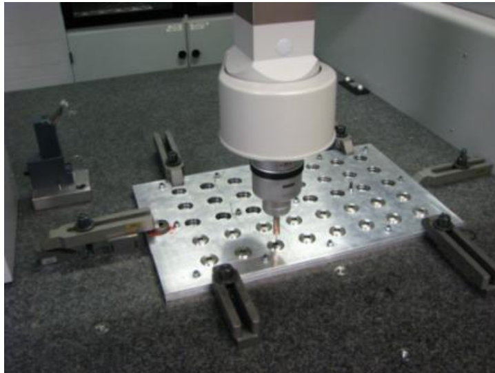
Fig. 4.6 - Fixture clamped to the CMM table
