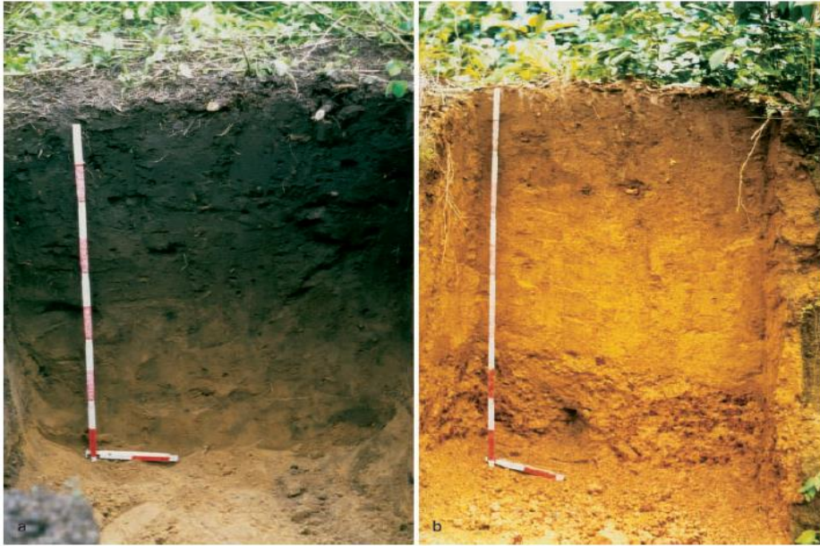
Figure 1.2 Comparison between Terra Preta from Amazonian forests (left; Anthrosol with high quantity of charcoal) and naturally soil Oxisol (right) [15].
