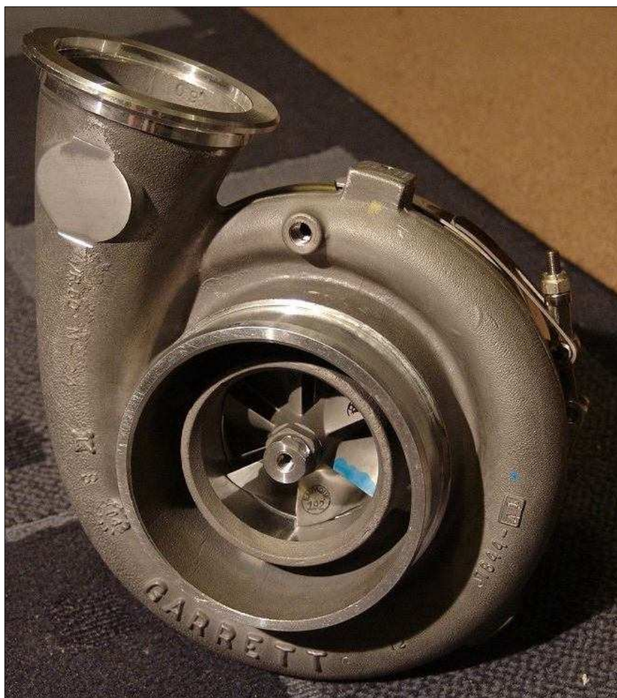
Obr 6.1 Volené turbodmychadlo GT4202R [21]
