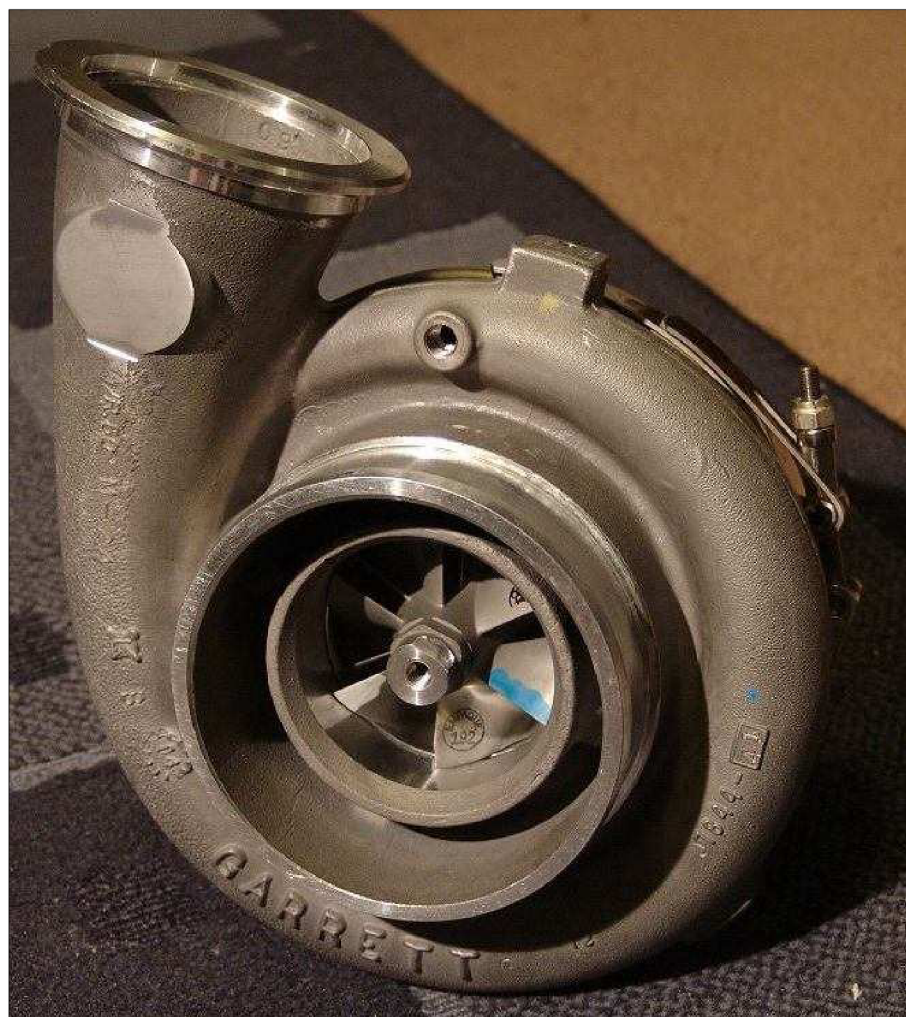
Obr 6.1 Volené turbodmychadlo GT4202R [21]
