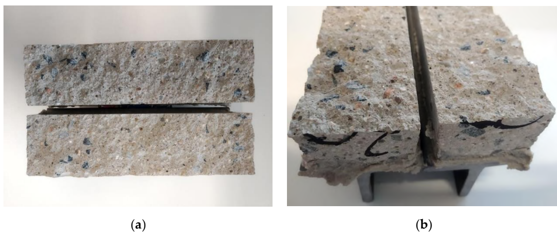
Figure 10. Failure of the specimens on the layer interface. (a) upper view; (b) detail view.
