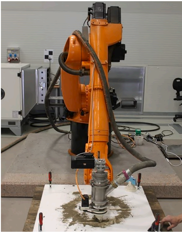
Fig. 1. Hose routing issues in the robotic arm.
