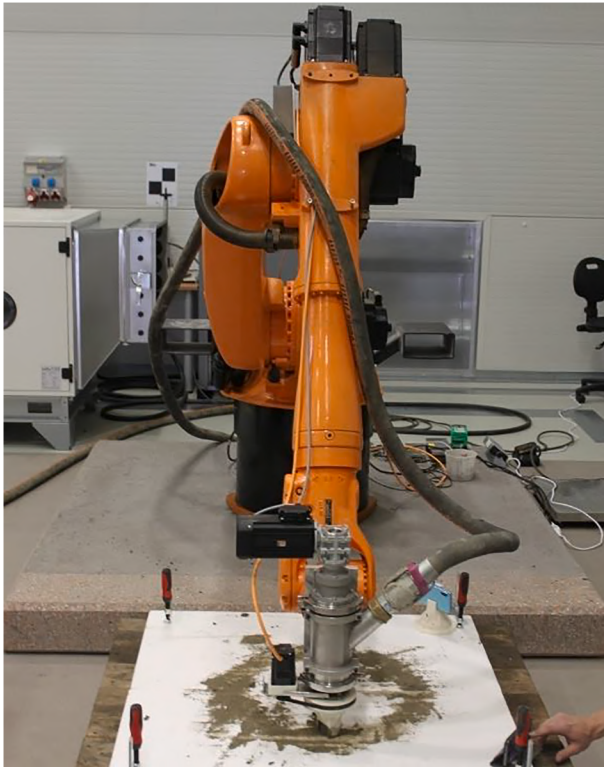
Fig. 1. Hose routing issues in the robotic arm.
