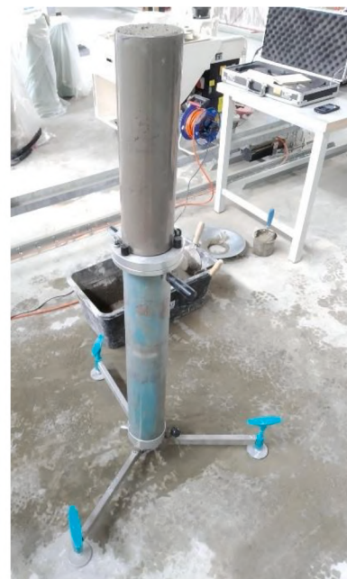
Fig. 2. Pipe rheometer: schema of a rheometer (a) and field test (b).
