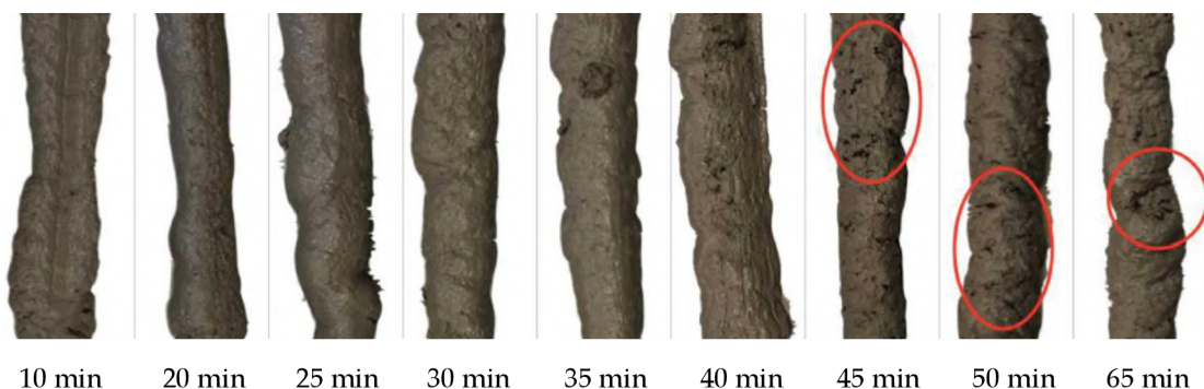
Figure 6. Quality of the single-layer extrusion: observation of the fluid consistency of extrusion from 10 min after mixing and crack occurrences from 45 min after mixing.
